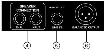
**4. SPEAKER THRU AND SPEAKER INPUT:** These are 1/4" mono phone jacks. When using an amplifier, the output from the power amp section connects to the 'speaker input' jack while the amplifier speakers connect to the 'speaker through' jack.
